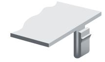
Figure 5. U-shaped snap-fit
