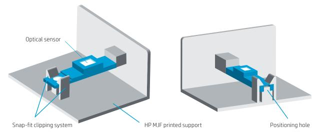
Figure 24. Optical sensor clipping system
