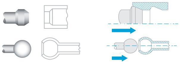
Figure 7. Annular snap-fit
