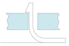
Figure 4. L-shaped snap-fit assembly operation
