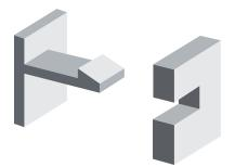
Figure 1. Cantilever snap-fit
