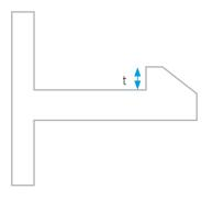
Figure 15. Minimum overhang depth (t)
