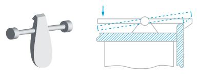
Figure 9. Torsional snap-fit
