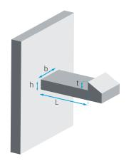
*Figure 11. Snap-fit geometry*
