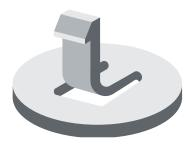
Figure 3. L-shaped snap-fit
