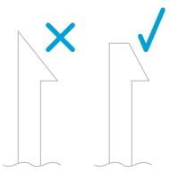
Figure 17. Snap-fit overhang
