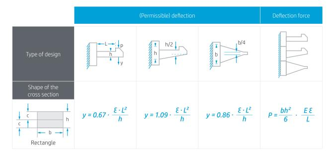
Figure 13. Snap-fit calculation equations\*
