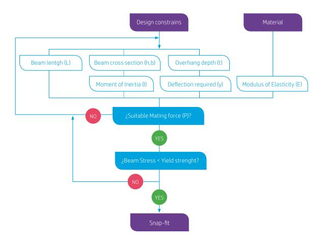
Figure 12. Design snap-fit flowchart
