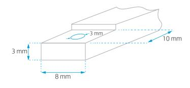
Figure 25. Optical sensor dimensions
